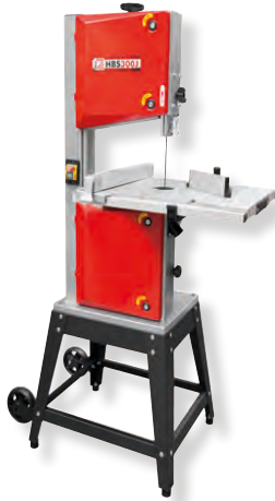
Räder am Untergestell wheels mounted on the stand
