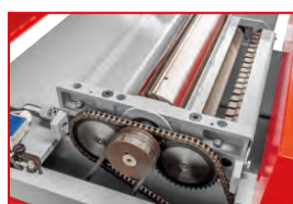
massiver Lagerblock solidly bedded cutter block
