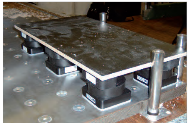
Innospann Steel-Plate-T | Retrofitting of a flat table with Steel-Plate-T, Mono-Bases and diverse suction cups, fixed on an intermediate plate
