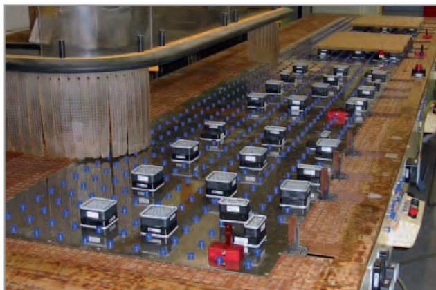
Innospann Steel-Plate | Retrofitting of a grid table with Steel-Plate, Mono-Bases and diverse suction cups
