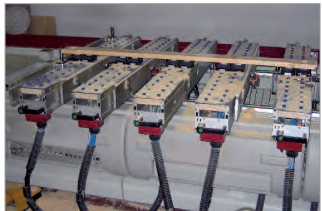
Innospann Steel-Plate | Retrofitting of a console table with Steel-Plate, Mono-Bases and diverse suction cups
