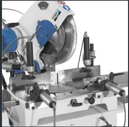
Pneumatic horizontal clamp (**T50 - T 53**) Pneumatic vertical clamp (**T50 - T 53**)
