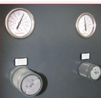
Regulators to adjust the vertical and horizontal thrust
