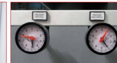
Hydraulic regulation of the vertical/horizontal thrust (Optional)
