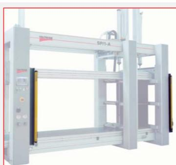
Photoelectric safety barrier (option)
