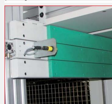
Third pair of horizontal pressure bars with auto positioning by ultra-sound sensor (option)
