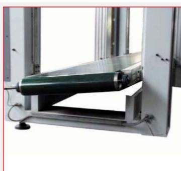
Tilting belt to ease the replacement of the belt
