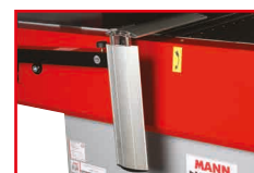
klappbare CPS Hobelwellenabdeckung CPS cutter block protection
