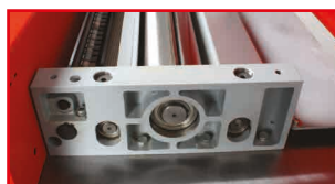
massiver Lagerblock solidly bedded cutter block
