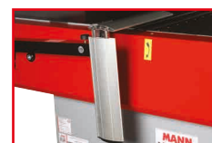
klappbare CPS Hobelwellenabdeckung CPS cutter block protection
