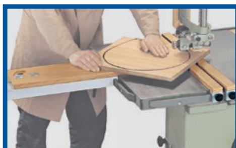
Kreisfix in combination with table extension to cut round work pieces
