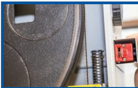
vulcanised-on rubber lining, spherically ground
