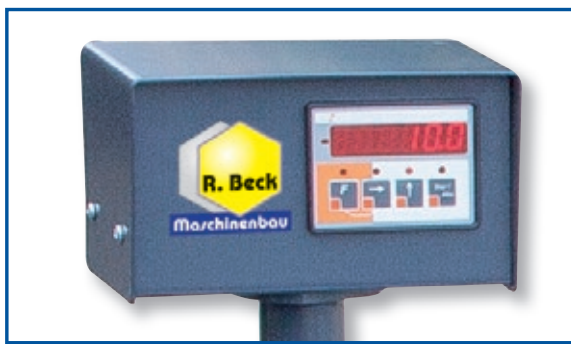
Indicator Z 58 with 0.1 mm display Input signal via magnetised pole ring and sensor head at the drive shaft item no. SZ 09
